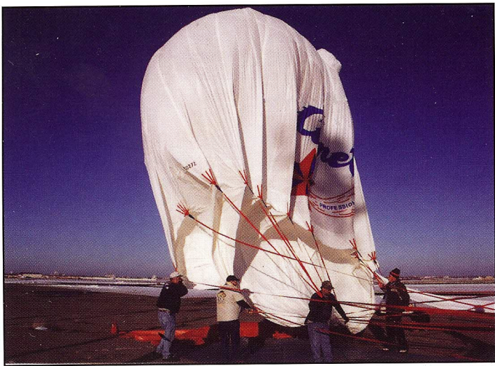
With load tapes singing in the 12-15 knot winds the crew struggles to inflate the 14,000 cu.ft. envelope.
